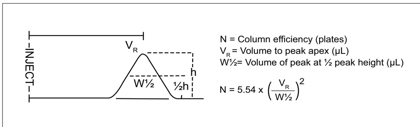
Figure 2. Half height method test calculations
