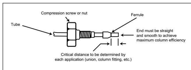
Figure 1. Ferrule and compression screw assembly
