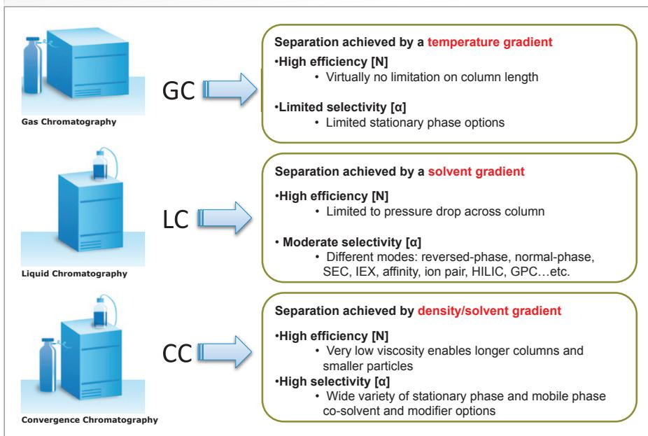
**Figure 2:** Evolution of SFC Instrumentation: ACQUITY UPC<sup>2</sup>.
