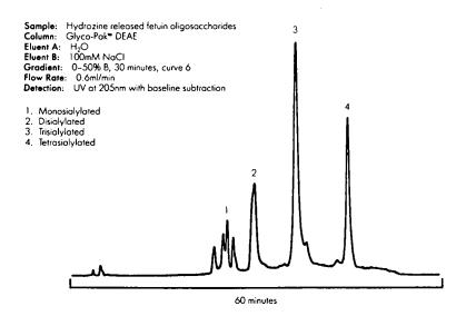
Oligosaccharides released chemically or enzymatically can be purified on the Glyco-Pak columns. Samples such as the Genzyme/Waters high mannose oligosaccharide standard can be purified in a single step.
