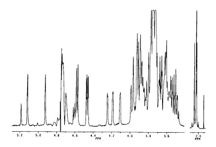
Structural reporter regions of 500-MH, proton NMR of peak 5 of neutral oligosaccharide standard, a biantennary structure with terminal galactose (from fibrinogen) after purification on the Glyco-Pak N column.
