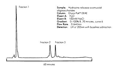
The initial fraction of oligosaccharides derived from ovomucoid is performed on the Waters Glyco-Pak DEAE column. Fraction 1 contains neutral carbohydrates and fractions 2 and 3 contain acidic carbohydrates.
