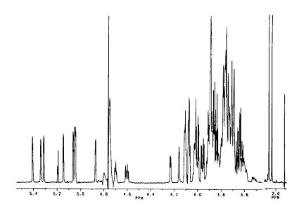
Structural reporter regions of  $500\text{-MH}_{z}$  proton NMR of peak 6 of neutral oligosaccharide standard, (Man 9 from soybean agglutinin) after purification on the Glyco-Pak N column.
