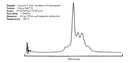
Fraction C collected from the Waters Carbohydrate Analysis column is now fractionated on the Glyco-Pak N column. This column provides an additional mode of separation with selectivity that is distinctly different from traditional NH<sub>2</sub> columns.
