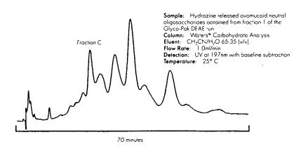
The neutral oligosaccharides obtained from fraction 1 of the DEAE run are now fractionated on the Waters Carbohydrate Analysis column.
