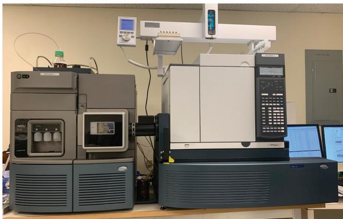
SGS AXYS scientists tested the capabilities of the APGC-MS/MS technology with the Waters Xevo TQ-XS Triple Quadrupole Mass Spectrometer.
