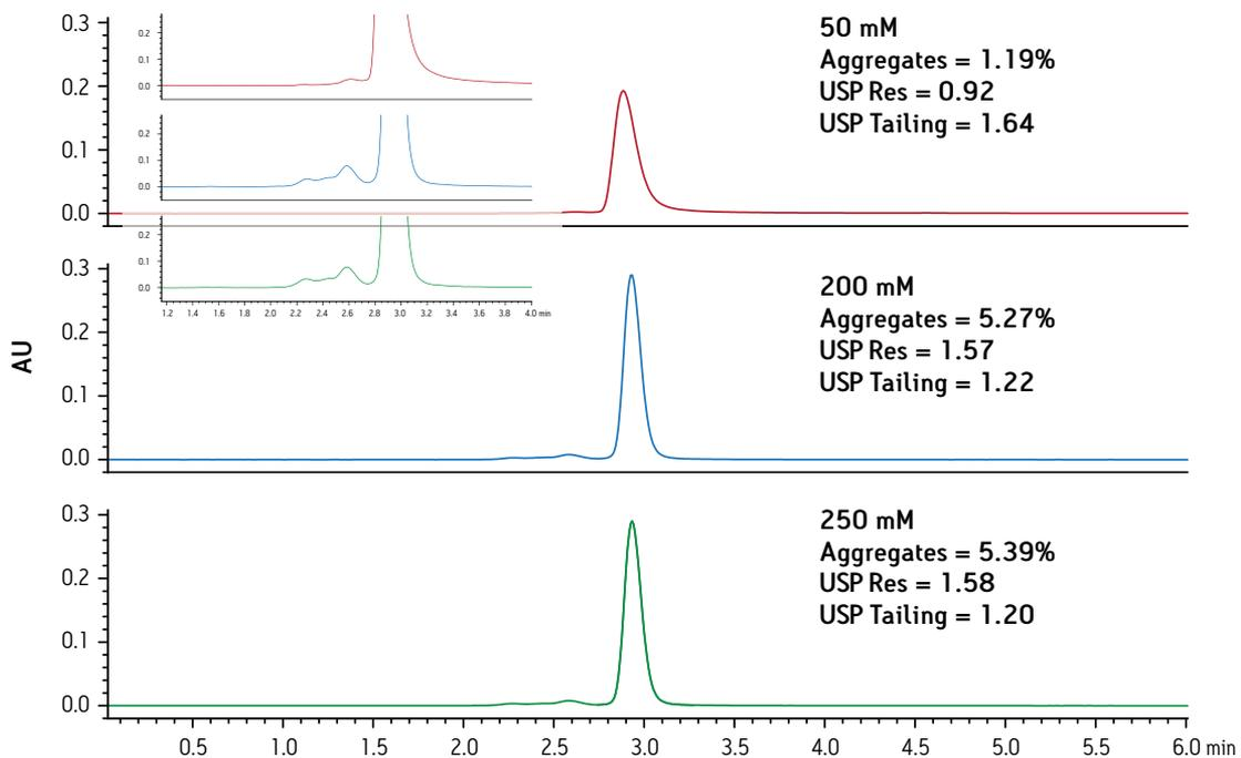
Figure 2. Effect of sodium chloride on the SEC separation of a murine mAb.
