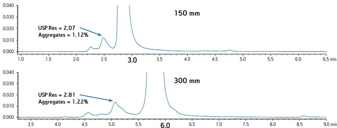
Figure 7. Effect of column length on a SEC separation of murine mAb.
