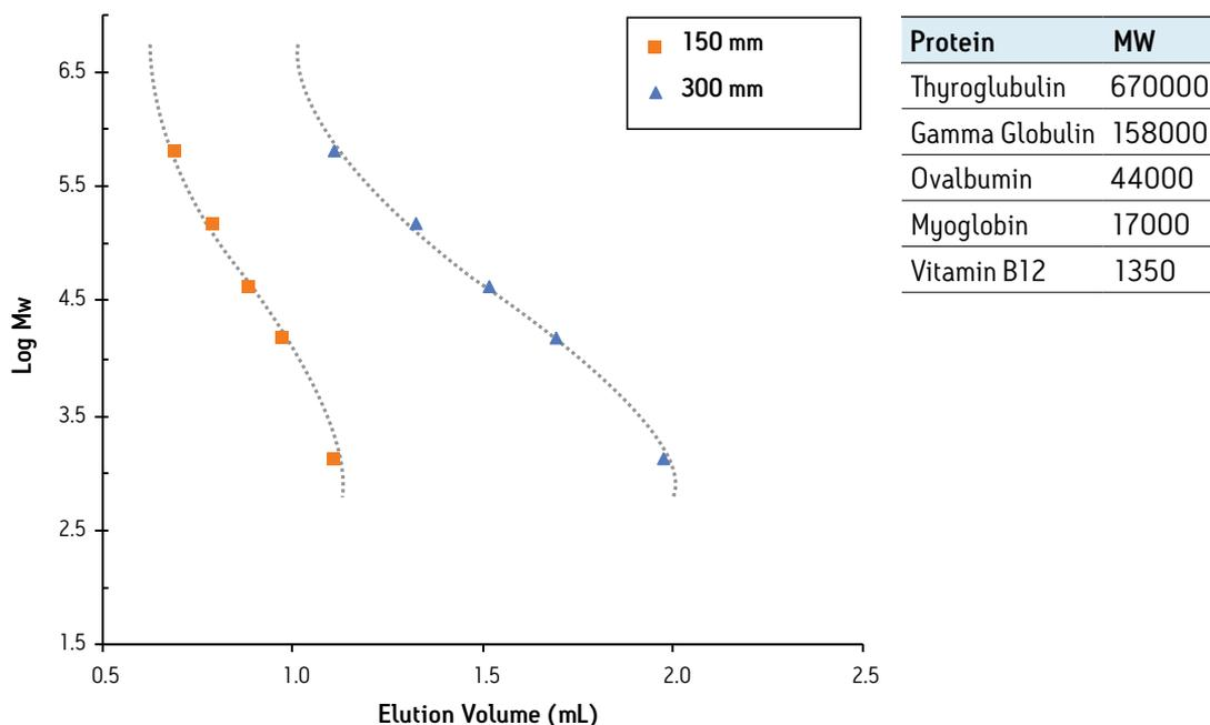
Figure 6. Effect of column length on SEC calibration curve.
