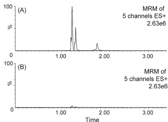
Fig. 3. TICs of MRM transitions for five phospholipids remaining in Elute 2 from mixed-mode cation exchange SPE using (A) basified methanol and (B) basified acetonitrile as the elution solvent. UPLC<sup>®</sup>/MS/MS with pH 9 mobile phase.
