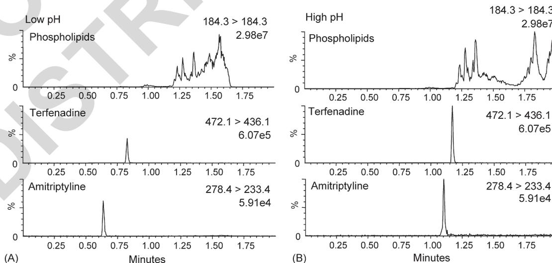
Fig. 4. MRM transitions for all phosphatidylcholine-containing phospholipids (top) from plasma samples prepared by ACN PPT analyzed by UPLC<sup>®</sup>/MS/MS under (A) pH 2.7 and (B) pH 9 mobile phase conditions. MRM transitions for 1 ng/mL terfenadine (middle) and amitriptyline (bottom) under the same mobile phase conditions.
