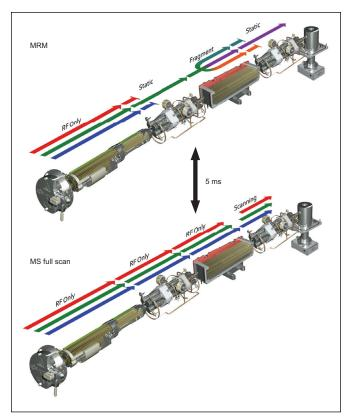
Figure 1. Xevo TQD ion path showing MRM and MS full scan mode acquisition.
