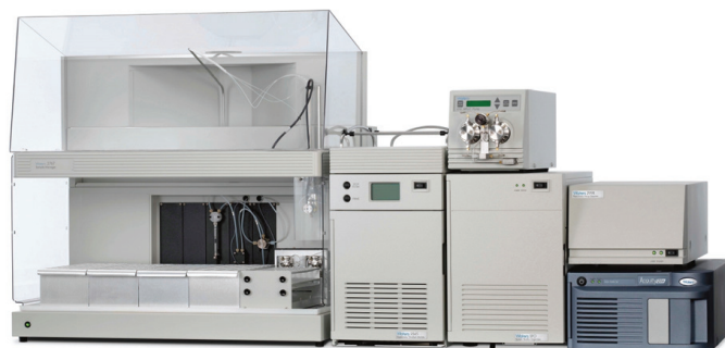
Figure 1. Waters AutoPurification System.
