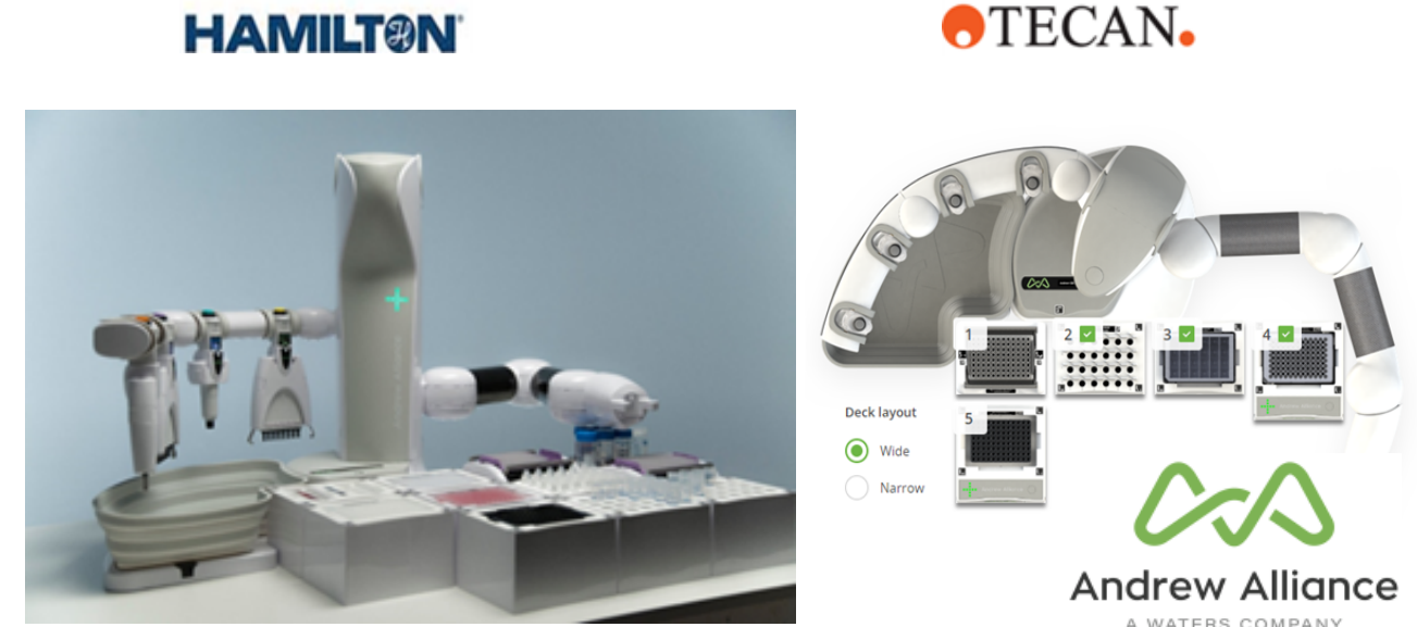
Figure 2: Amino acid analysis automation platforms: Tecan, Hamilton, and Andrew +
