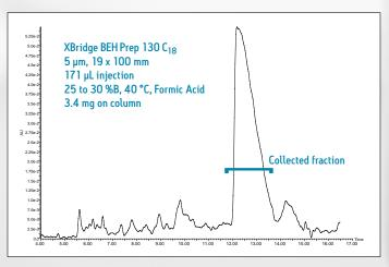
The separation is then scaled to a larger HPLC column for peptide isolation and fraction collection.
