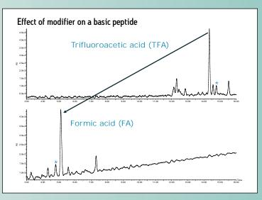
Selectivity can be altered to improve yield and purity by changing the modifier; in this example, good peak shape is maintained with both modifiers with a Peptide Separation Technology Column.
