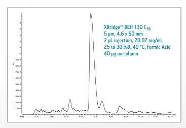
Using a focused gradient, the UPLC separation is transferred to an HPLC preparative system to expand the separation.
