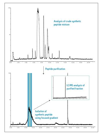
In a typical purification procedure, the crude synthetic peptide mixture is first analyzed and then the bulk of the impurities are removed with a Waters Purification System. A fraction highlyenriched in the desired peptide is obtained.
