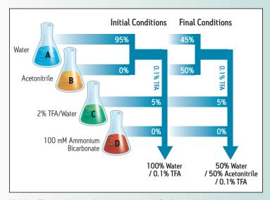
With  $Auto \bullet Blend$ , gradients can be generated automatically. Here, methods can be switched from low pH to high pH by selecting modifiers C or D.
