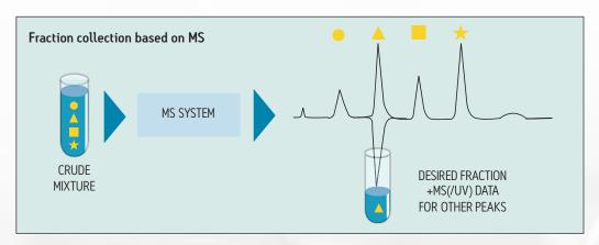
An MS detector can simplify the isolation process by tracking the product peptide. In the analytical run shown, the need to trigger on mass is evident since there is no definitive peak in the UV trace. This particular peptide has no strong chromophores.
