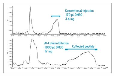
At-Column Dilution can allow five-fold or greater increase in the amount of peptide that can be isolated in a single injection.
