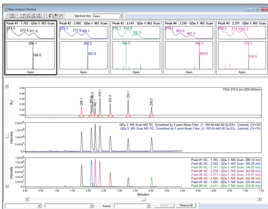
Figure 5. Empower 3 Software provides a view of mass and UV chromatograms and spectra. The UV chromatogram can be labeled with most intense ion at the peak apex. This view provides the tools for streamlined peak tracking and identification of coeluting peaks.
