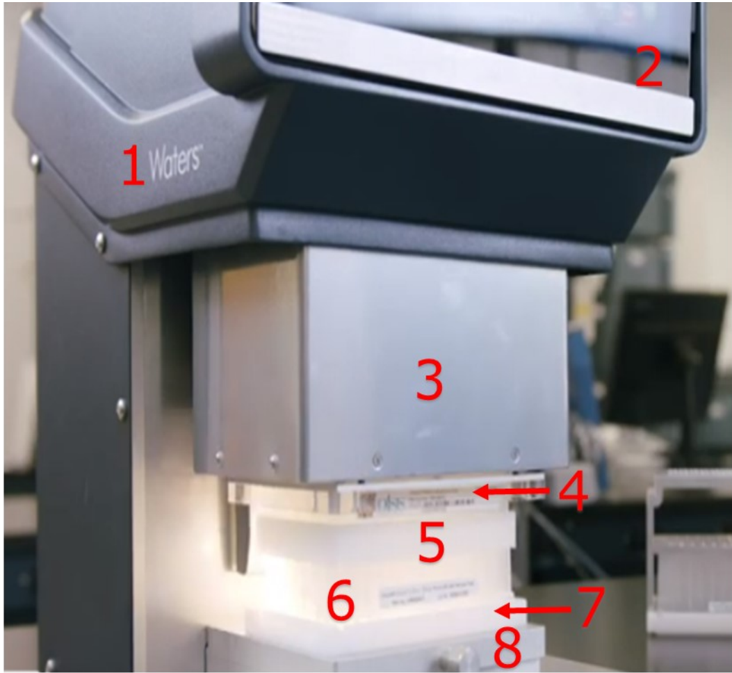
Figure 4. Otto SPEcialist Manifold Layout for oligonucleotide sample extraction using Oasis WAX µElution SPE. The use of this semi-automated device will allow for even pressure applied across every well of the plate.
