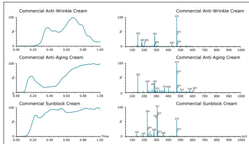
Figure 1. The complex sample spectra were recorded for the bulk sample without dilution, extraction, or any sample pre-treatment. Note that both negative and positive ionization were collected – positive ionization data are displayed.
