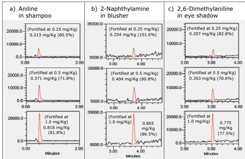
Figure 3. SIR chromatograms for selected PAAs in matrix: a) shampoo b) blush, and c) eyeshadow.
