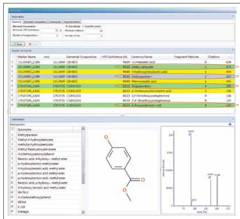
Figure 5. Discovery tool results for  $m/z$  151.0409 and 179.0724. Summary of elemental compositions, citations for structures retrieved from ChemSpider database and a number of possible fragment matches in high collision energy data for each structure.
