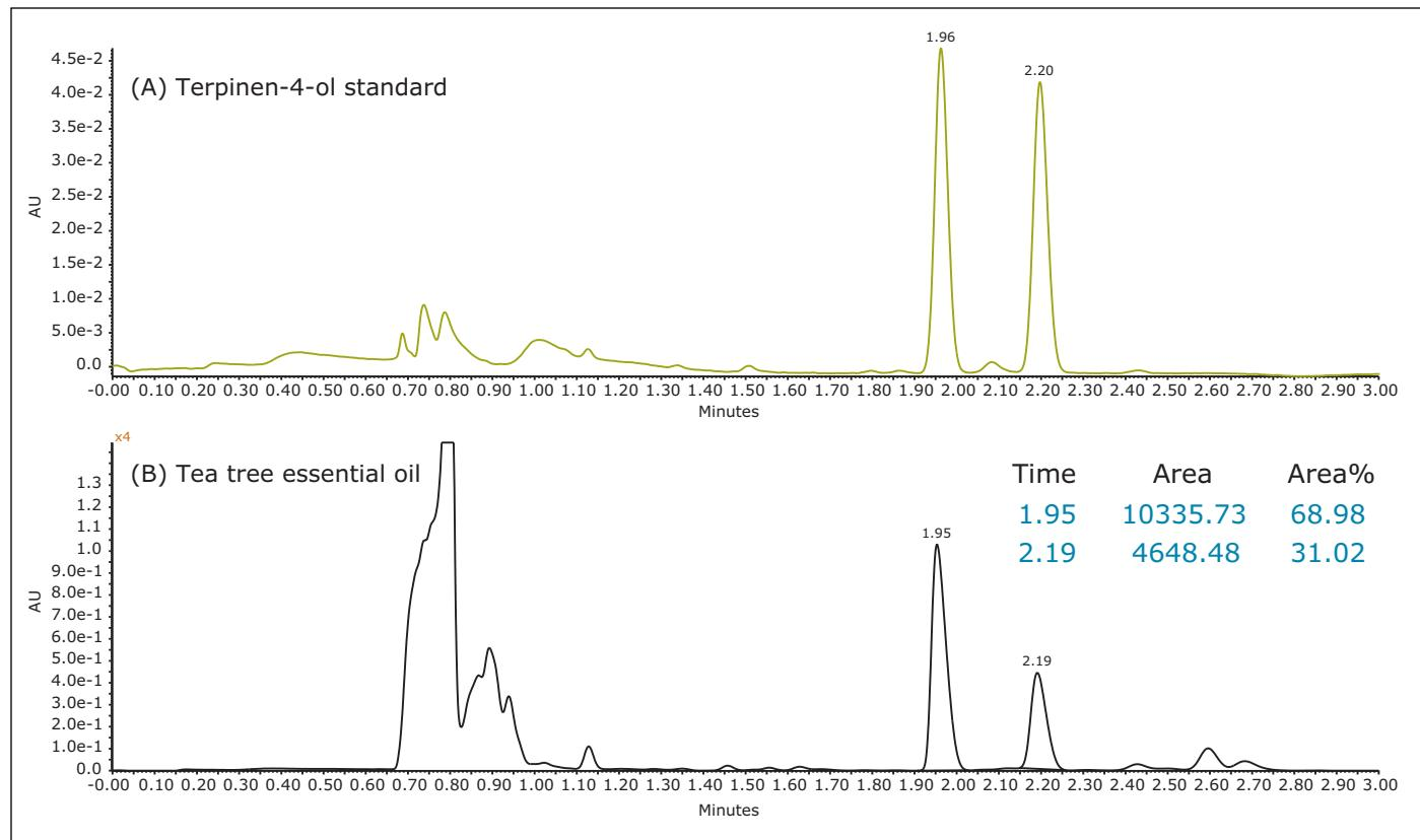
Figure 4. UPC<sup>2</sup>-UV chromatograms of (A) Terpinen-4-ol standard and (B) Tea Tree essential oil on an ACQUITY UPC<sup>2</sup> Trefoil AMY1 column. An isocratic method with 5% isopropanol was used. The flow rate was 1.0 mL/min.
