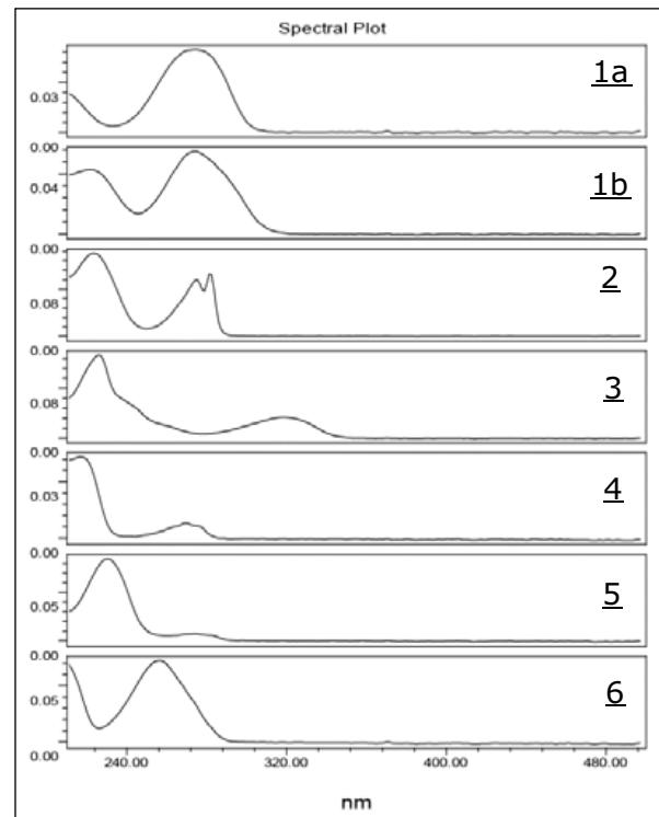
Figure 4. UV spectra of 1a, 1b, and 2–6 extracted from PDA data.
