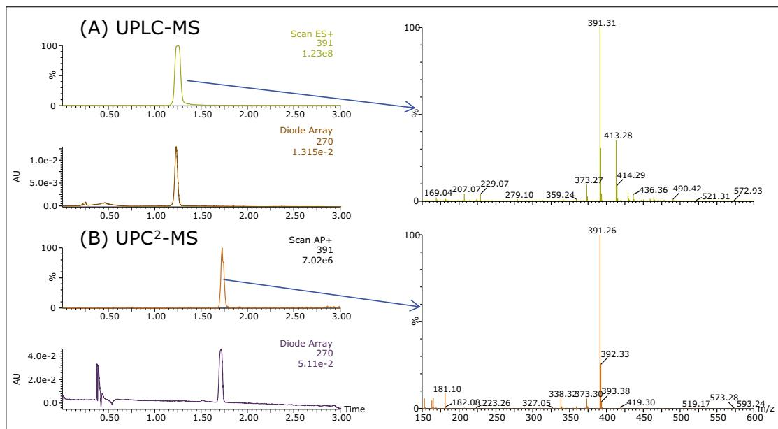
Figure 6. Purity analysis of the final product by (A) UPLC-MS and (B) UPC<sup>2</sup>-MS.
