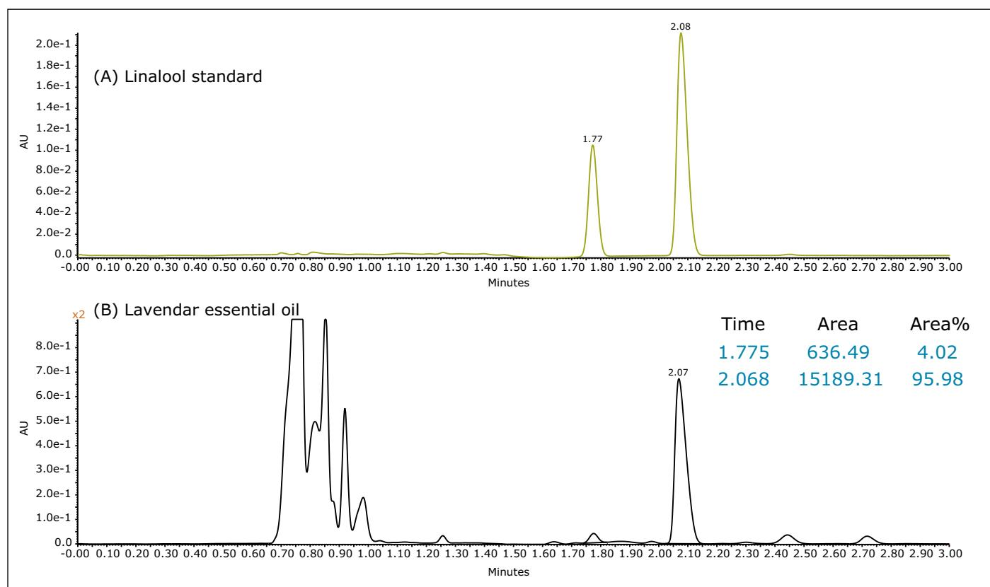
Figure 3. UPC<sup>2</sup>-UV chromatograms of (A) linalool standard (B) lavender essential oil on an ACQUITY UPC<sup>2</sup> Trefoil AMY1 Column. An isocratic method with 3% isopropanol was used for linalool. The flow rate was 1.0 mL/min.
