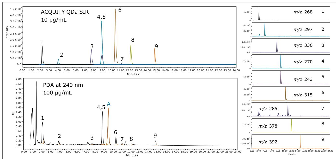
Figure 2. ACQUITY Arc chromatogram from the separation of nine disperse dye standards (100  $\mu$ g/mL, 5  $\mu$ L injection) at 240 nm using the DIN 54231 standard method and an XBridge C<sub>18</sub>, 2.1 x 150 mm, 5.0- $\mu$ m Column (lower). The superimposed (top) and the individual stacked (right) SIR channel chromatograms (10  $\mu$ g/mL, 5  $\mu$ L injection) are also shown.
