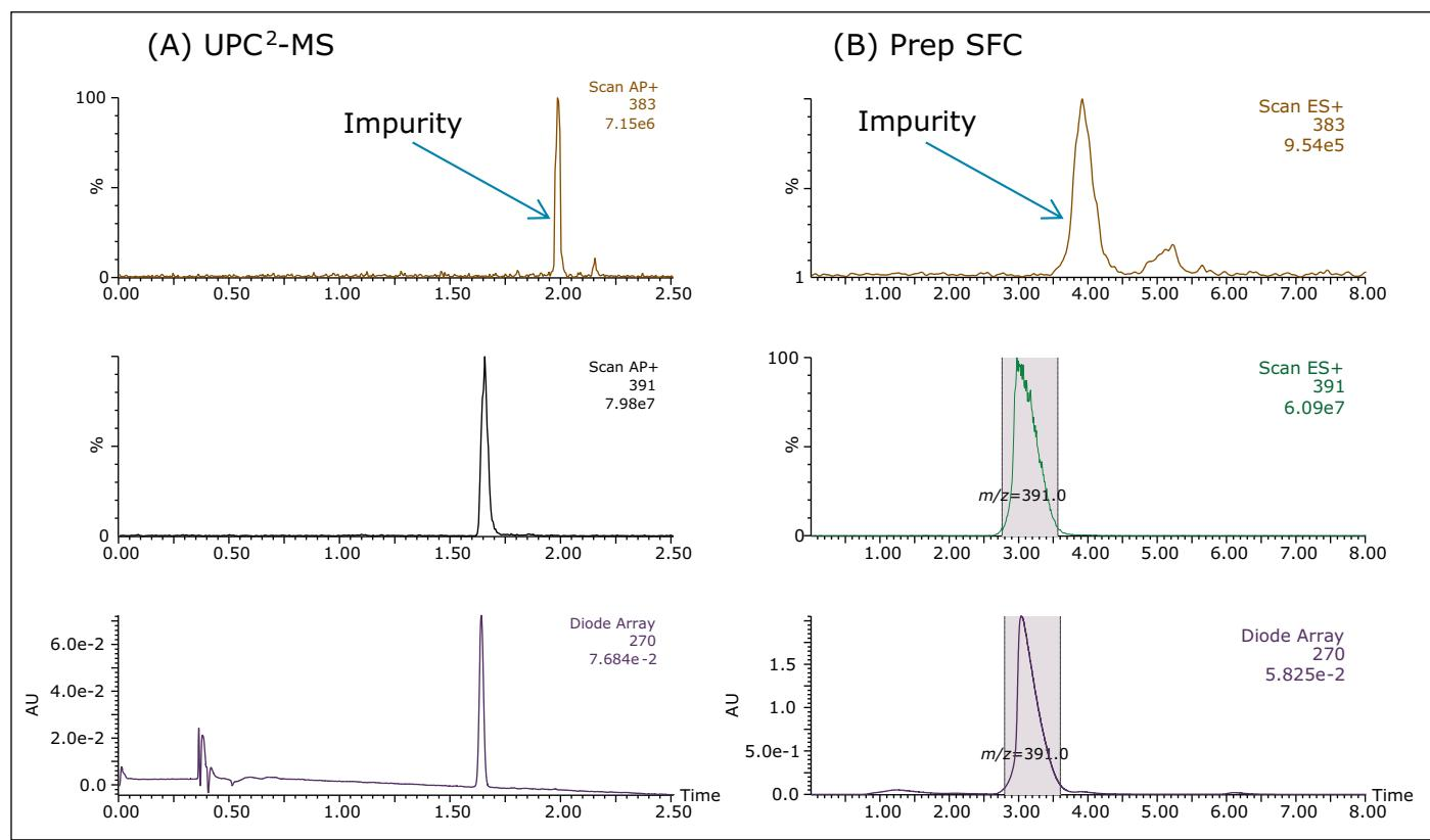
Figure 3. (A) UPC<sup>2</sup>-MS and UV chromatograms of the MPLC fraction at 1 mg/mL; and (B) prep SFC-MS and UV chromatogram of the MPLC fraction at 20 mg/mL.
