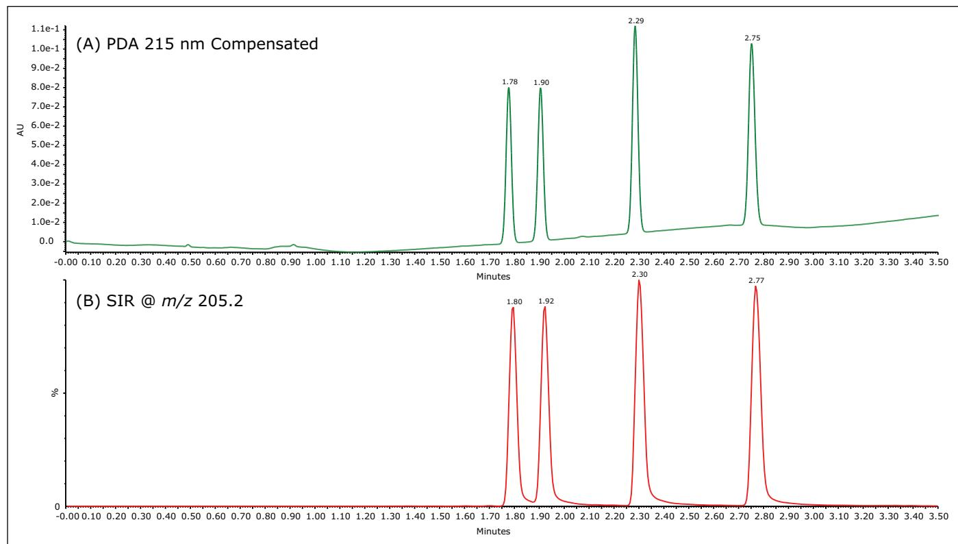
Figure 5. UPC<sup>2</sup> chromatograms of a nerolidol standard separated on an ACQUITY UPC<sup>2</sup> Trefoil AMY1 Column: (A) UV at 215 nm with a compensation wavelength of 260-310 nm; and (B) SIR at  $m/z$  205.2. The flow rate was 1.5 mL/min. A gradient of 2-7% isopropanol in 3.5 min was used.
