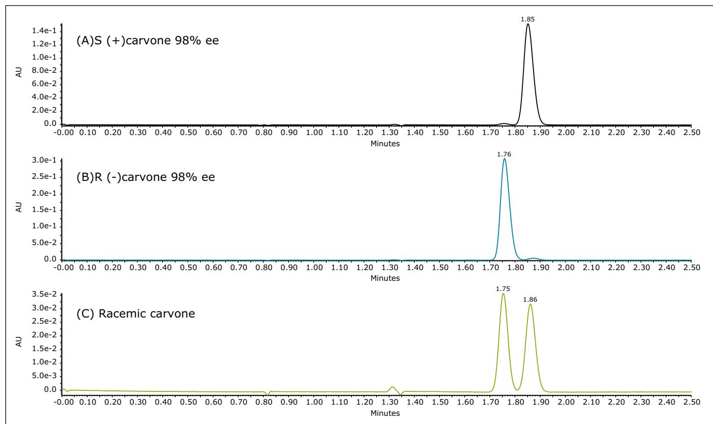
Figure 2. UPC<sup>2</sup>-UV chromatograms of the enantiomeric separation of carvone on an ACQUITY UPC<sup>2</sup> Trefoil CEL1 Column: (A) S (+) carvone; (B) R (-) carvone; and (C) racemic carvone. An isocratic method with 4% isopropanol was used. The flow rate was 0.9 mL/min.
