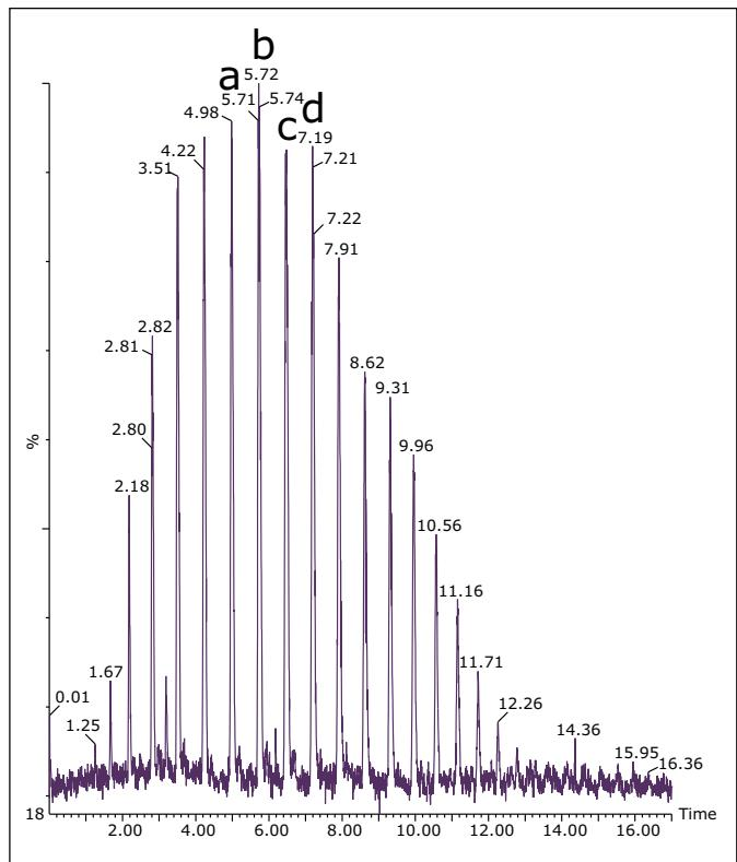
Figure 3. MS chromatogram for a Triton X-100 standard.
