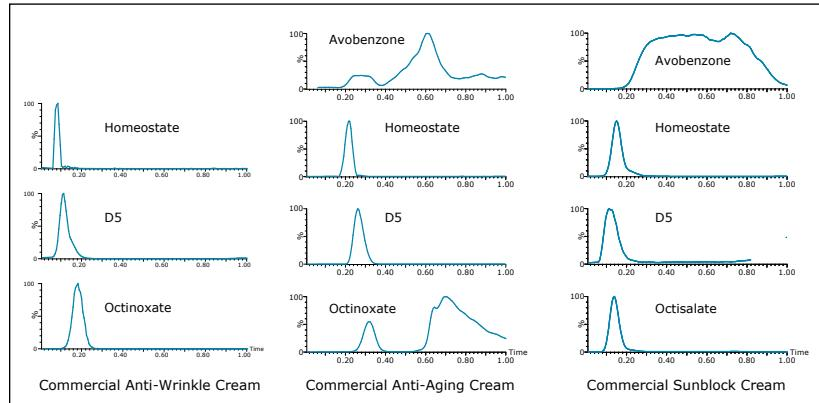
Figure 2. Thermal desorption chromatograms for the target analyte list using MS/MS data. Each thermal chromatogram was processed using a simple smoothing function to provide consistent data over the acquisition range.
