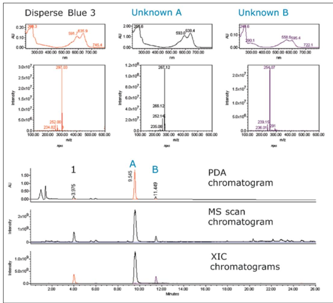
Figure 4. Empower Software's Mass Analysis window showing UV and MS spectra (top). ACQUITY Arc, PDA, MS scan (100–600  $m/z$ ) and superimposed XIC chromatograms of a single standard of disperse blue 3 using the DIN 54231 standard method.
