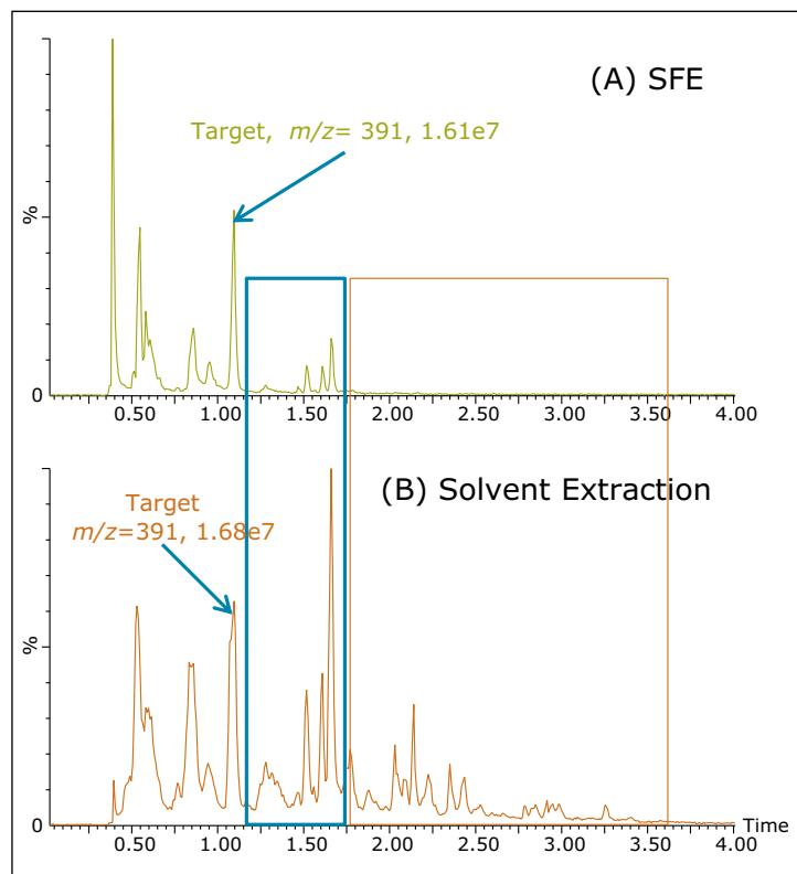
Figure 1. UPC<sup>2</sup>-MS chromatograms of the mixtures obtained by (A) SFE and (B) methanol extraction, using an ACQUITY UPC<sup>2</sup> 2-EP Column.
