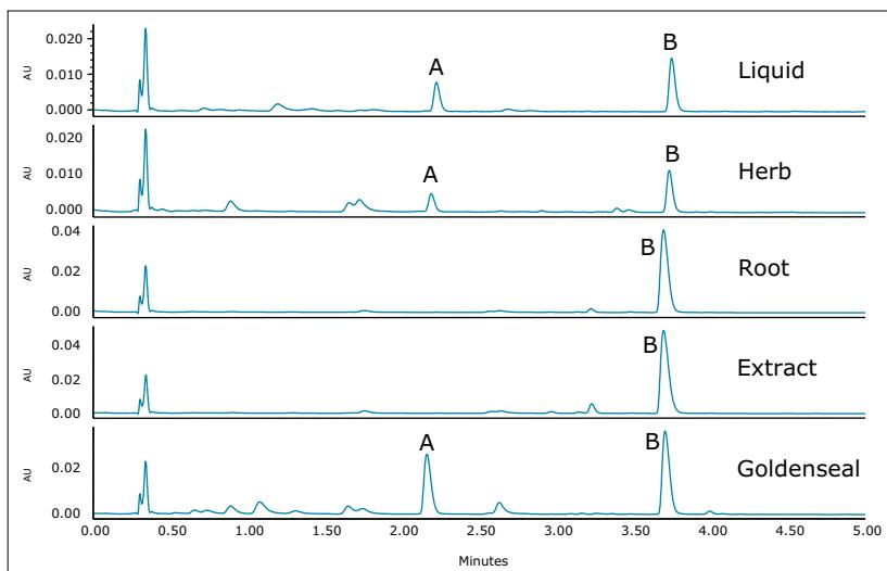
Figure 1. Separation of five different sources of Goldenseal on a CORTECS  $C_{18+}$ , 2.7  $\mu\text{m}$ , 3.0 x 50 mm Column at 300 nm. Main components A and B are indicated. Maximum pressure for the separation was 2600 psi.
