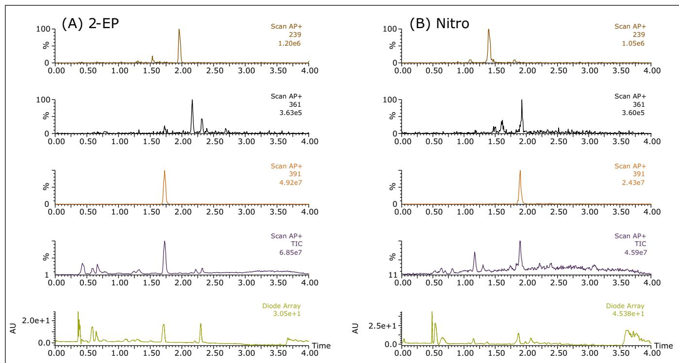
Figure 4.  $\text{UPC}^2\text{-MS}$  and UV chromatograms of the SFE extract using (A) a 2-EP; and (B) a nitro column.
