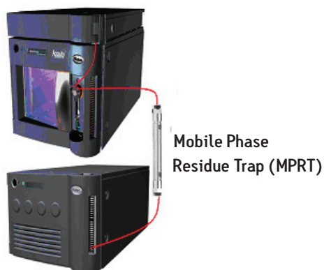
Figure 1. Modification of UPLC system to reduce the interference of mobile phase PFC presence.
