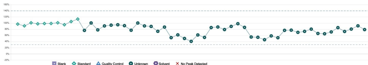
Figure 4. Plot extracted from MS Quan Application showing the trend of M8 PFOS used as a recovery standard, where all injections fell within the 30 to 140% tolerance (dotted blue lines) stated in the EURL for POPs guidance document.
