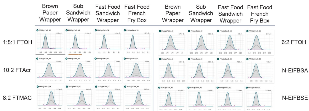
Figure 5. Example chromatograms showing overlaid quantitative and qualitative MRMs of selected PFAS spiked into food packaging materials at 25 ng/mL.
