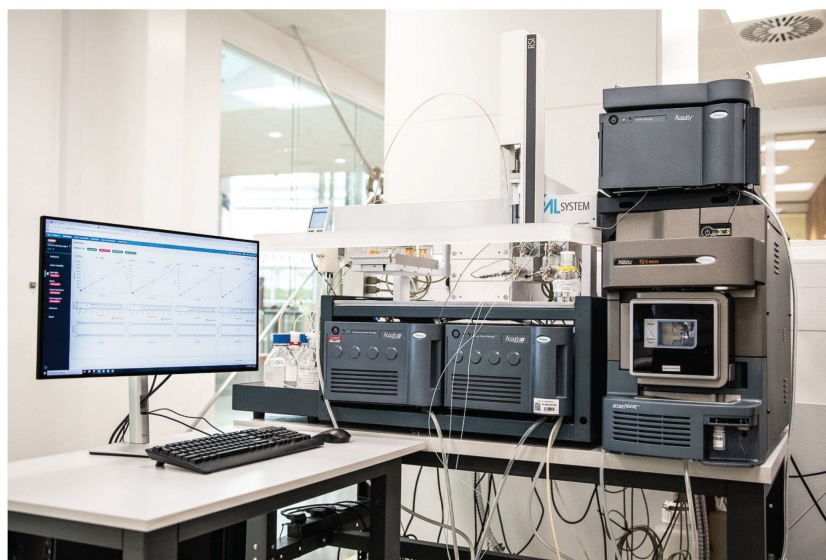
Figure 1. Automated Online SPE System including the CTC PAL RSi configured for 2D trap and elute coupled to Xevo TQ-S micro Mass Spectrometer with Unispray ionisation under waters_connect for Quantitation Software Control.
