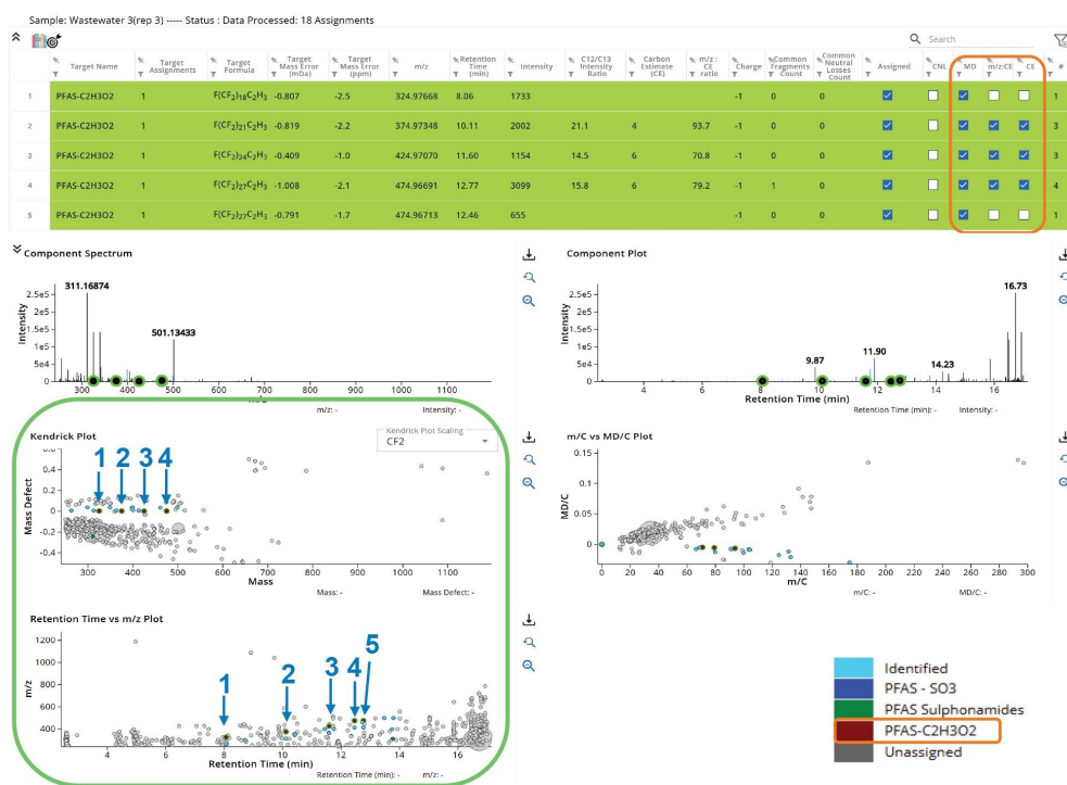
Figure 3. Combined table and component data visualization. The data was filtered with a threshold of 500 and using the mass defect filter. Light blue circles denote targets identified in UNIFI Software, and grey denotes unidentified components. Other colors denote the chemical component assigned.
