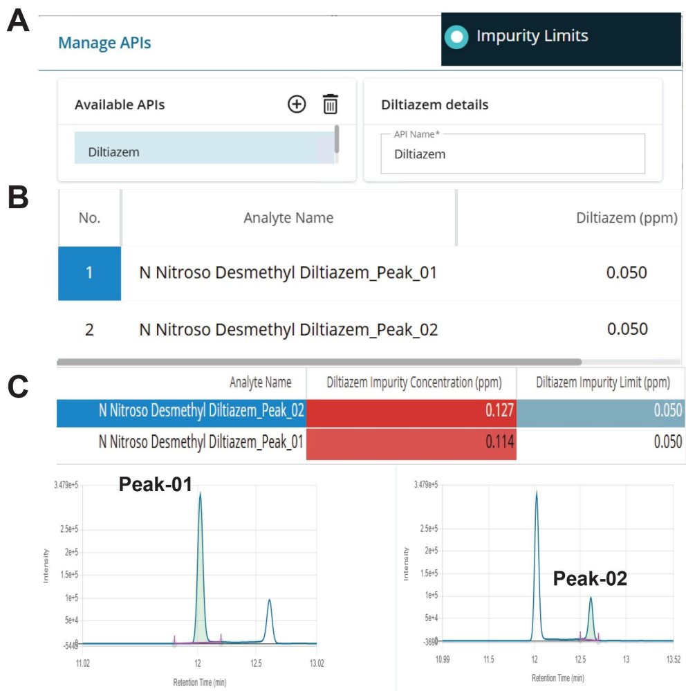
Figure 9. Diltiazem hydrochloride, API (A) the NDD impurity and the regulatory limits can be defined in MS Quan method (B) Quantitative impurity results from extracted tablet samples exceeding the specified limit of 0.05 ppm, flagged in red. (C) Chromatograms showing the detected impurity isomers are also displayed.
