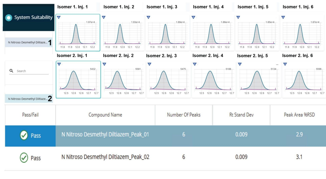
Figure 6. The system suitability feature can be enabled in the software to calculate the standard deviation of the retention time and the %RSD of the peak area for the analytes specified in the method. The LC/MRM chromatograms for each isomer injection ( n = 6 ) are also shown, 0.2 ng/mL, (0.005 ppm method equivalent).
