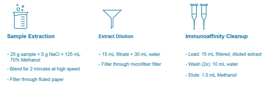
Figure 1. Representation of the sample preparation protocol for AOAC Official Method 991.31: Aflatoxins in corn, raw peanuts, and peanut butter: Immunoaffinity Column (AflaTest) Method.
