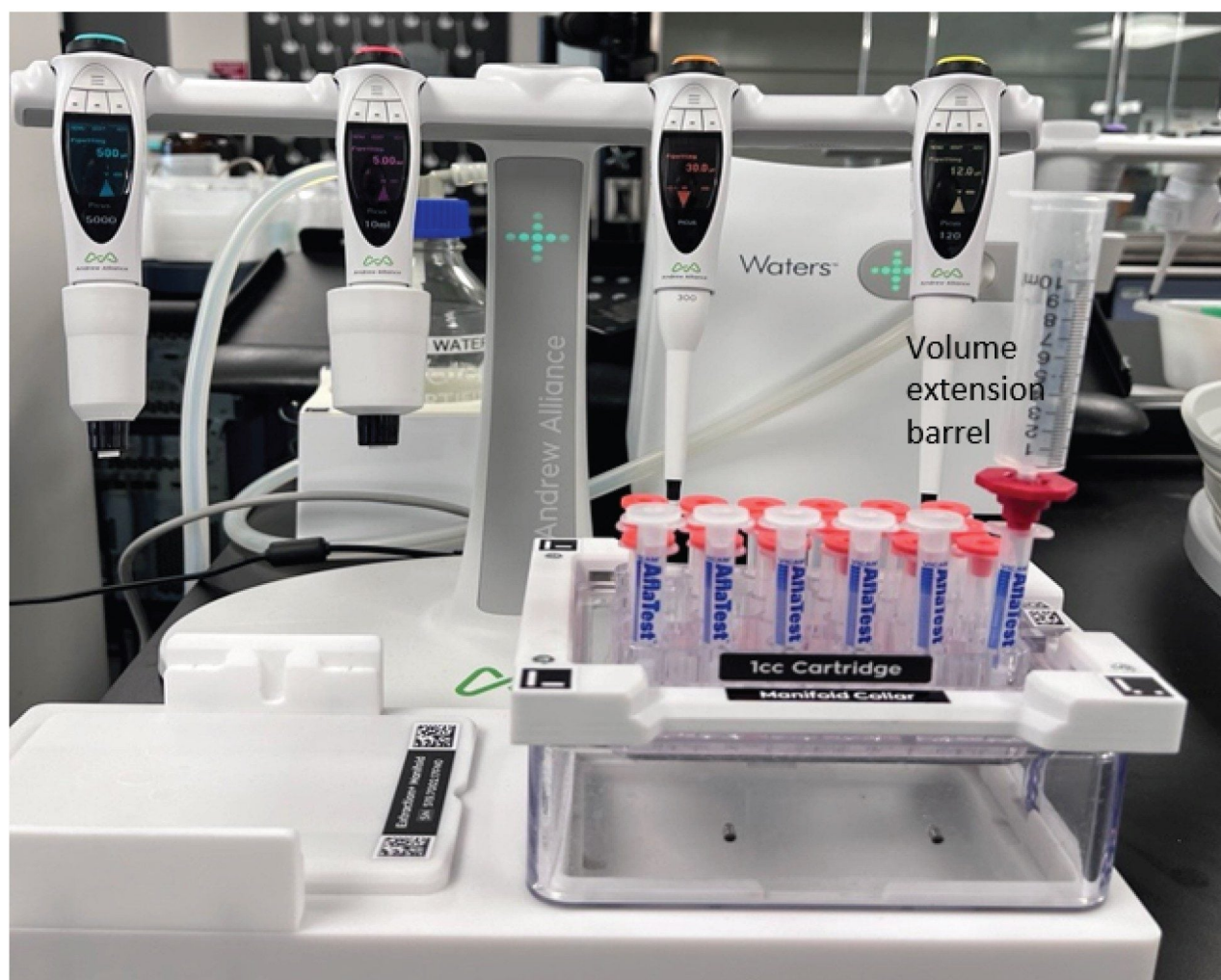
Figure 2. Compact setup allows cleanup of 24 samples at a time. A volume extension barrel is coupled to the cartridge to allow the entire sample to be loaded in a single step.
