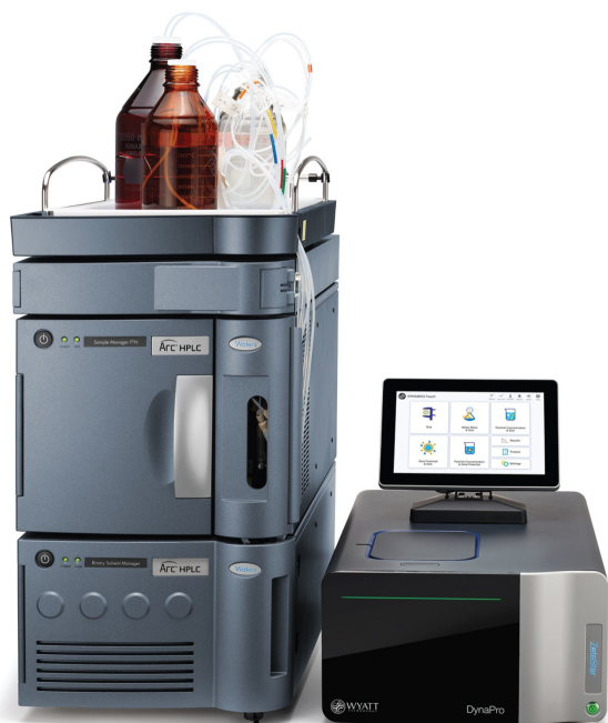
Figure 1. Waters Arc HPLC and DynaPro ZetaStar System.
