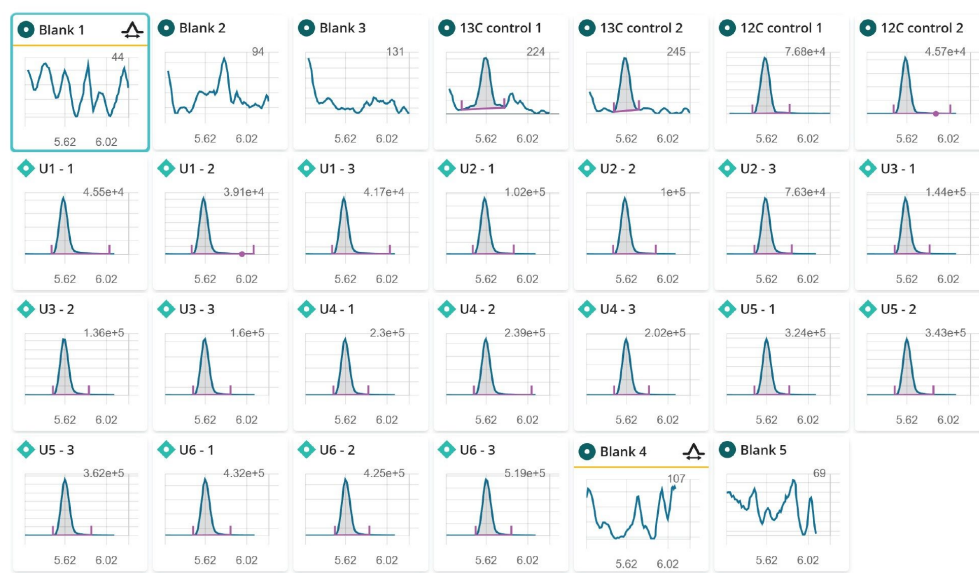
Figure 4. Data processing using the MS Quan Application within the waters_connect Software Platform showing the integrated chromatograms for L-methionine across all samples analyzed.
