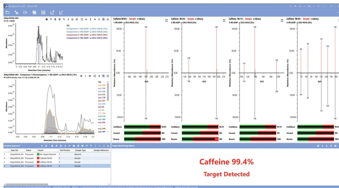
Figure 2. An example of the AnalyzerPro XD software results for seized sample #170. The upper panel shows the acquired spectra aligned with the corresponding cone voltage entries in the seized -drug spectral library, across all four cone voltages. The lower panel identifies caffeine as the predominant constituent, together with a match confidence of 99.4% following a ‘dip-and-detect’ analysis of the sample.
