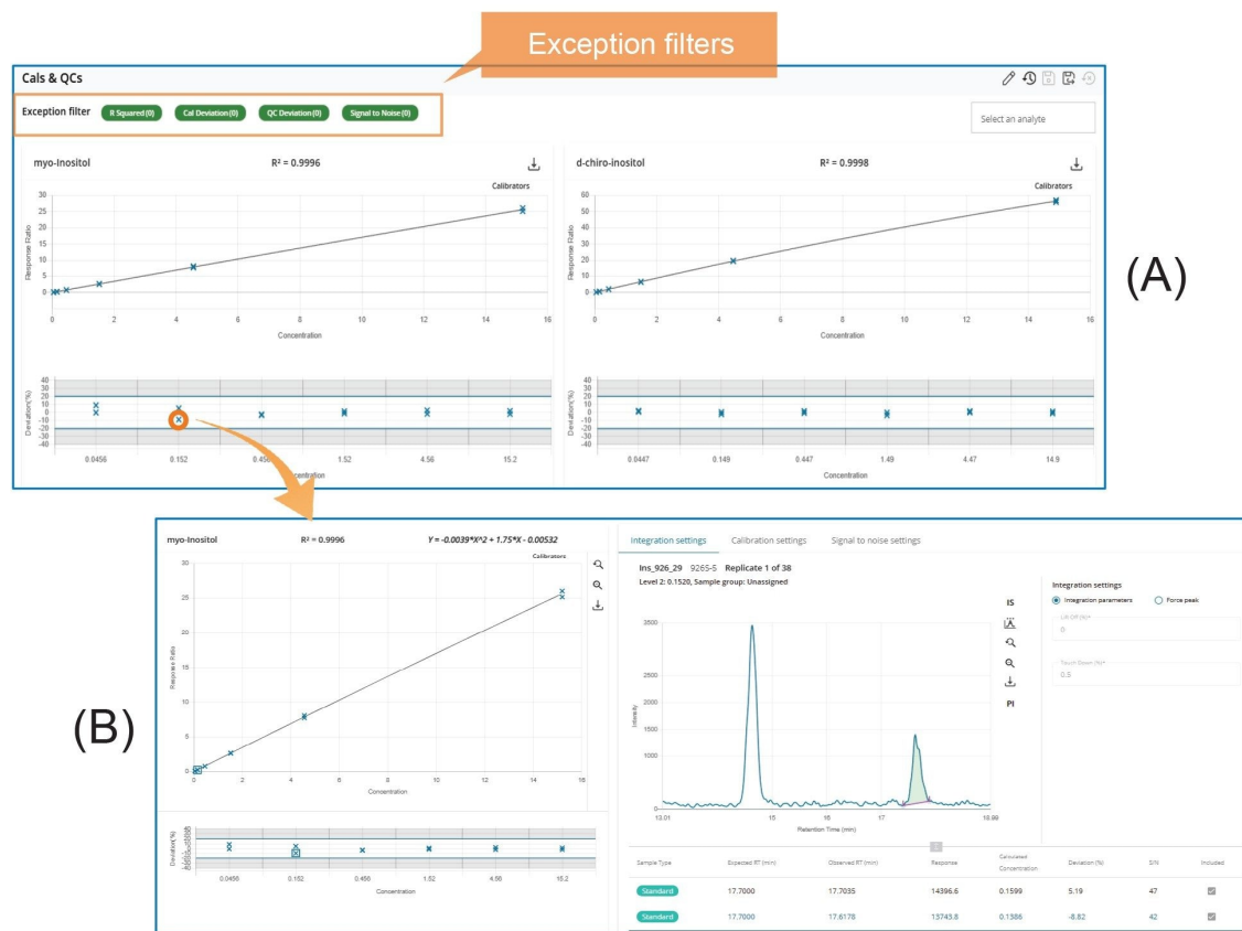
Figure 4. Screenshots of the Calibration Overview (A) and the individual calibration point review (B), accessible by clicking on a data point on the Overview page (indicated by the arrow). Exception filters are also highlighted on the Overview page.
