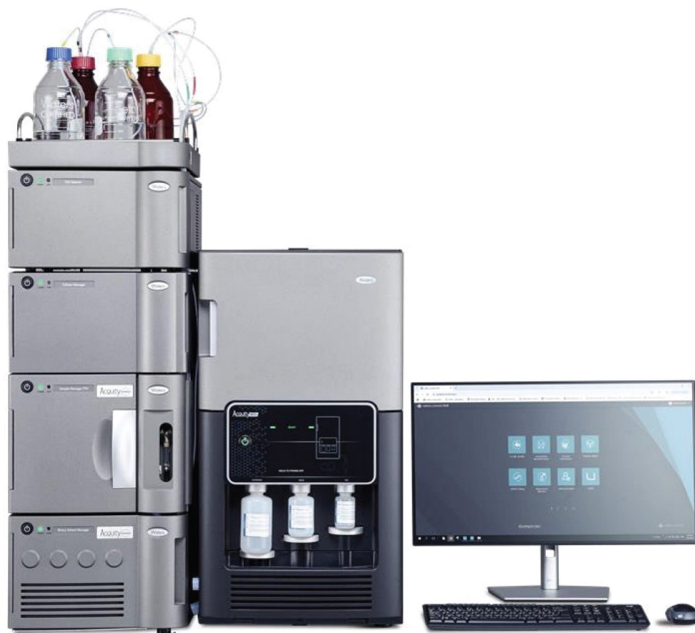
Figure 1. The BioAccord LC-MS System with ACQUITY™ Premier UPLC™ System, includes an ACQUITY Premier Binary UPLC System, tunable UV (TUV) detector coupled in-line with ACQUITY RDa™ Mass Detector, operated under the waters_connect Informatics Platform.
