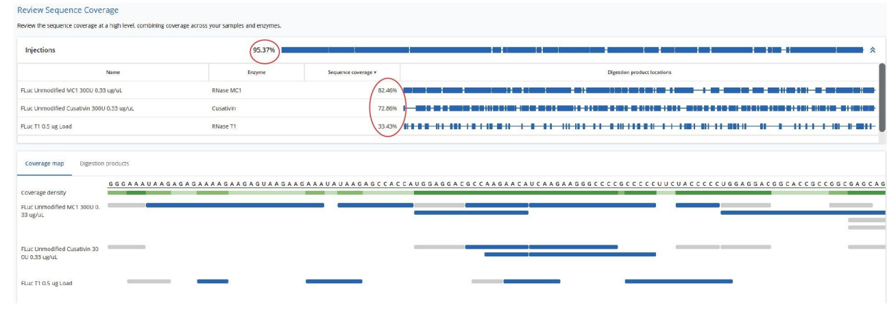
Figure 6. Comparison of sequence coverage obtained using MAP Sequence v2.0 for digestion of the Fluc mRNA with three enzymes, RapiZyme Cusativin, RapiZyme MC1, and RNase T1, assuming up to four missed cleavages. The combined sequence coverage demonstrates that the sequence coverage can be significantly increased through the multi-enzyme digestion approach outlined in this workflow.
