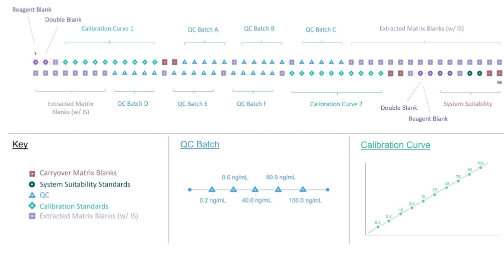
Figure 3. A visual guide to the run format for a 96-well plate used in this robustness experiment; each marker represents a unique plate well. Calibration and QC concentrations are detailed below the plate guide, alongside a color-coded key.
