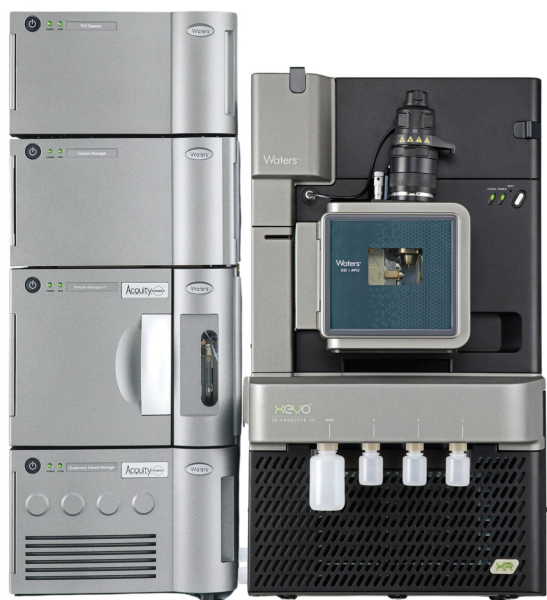
Figure 1. The Xevo TQ Absolute XR Mass Spectrometer and ACQUITY™ Premier LC System.
