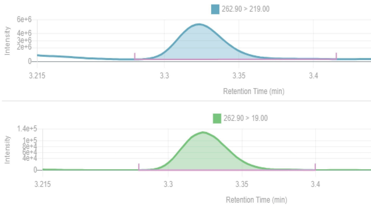
Figure 3. Quantitation (top) and Confirmation (bottom) MRM chromatograms for PFPeA in leachate.
