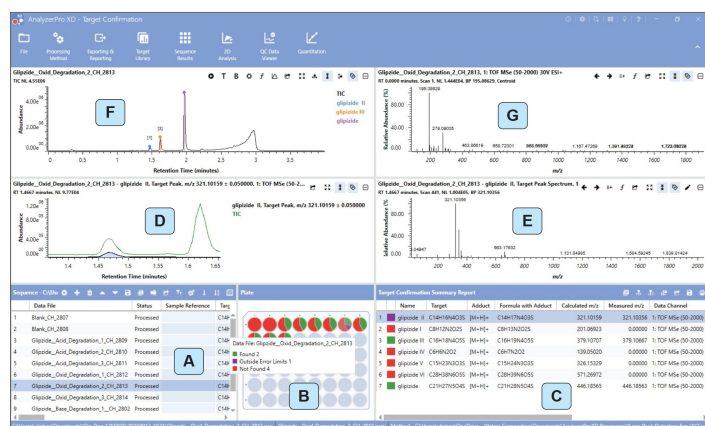
Figure 3. Data review in AnalyzerPro XD showing processed glipizide degradation data.
