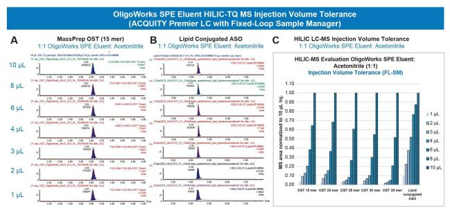
Analysis :ACQUITY Premier (Fixed-Loop Sample Manager 10 µL Loop with partial loop pressure assist ,Injection mode)-TQ Absolute MS Systems
