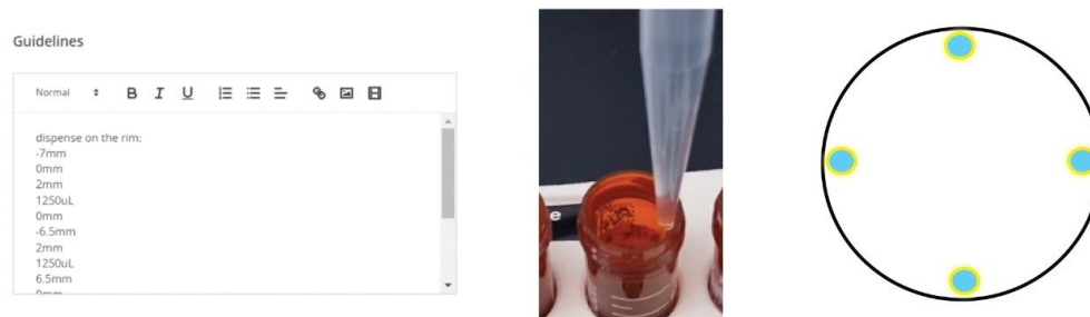
Figure 7. OneLab guidelines to dispense solvent along 4 positions of solvent dispensing (right).
