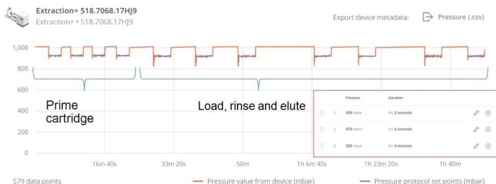
Figure 8. Programmable stepwise pressure gradient to ensure optimal flow through cartridges.
