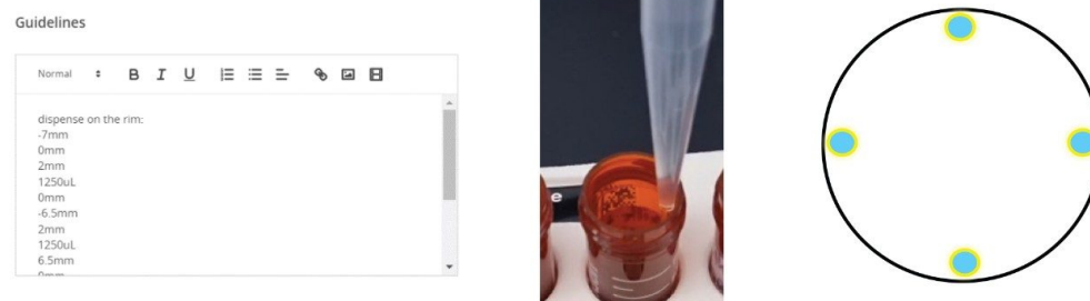
Figure 7. OneLab guidelines to dispense solvent along 4 positions of solvent dispensing (right).
