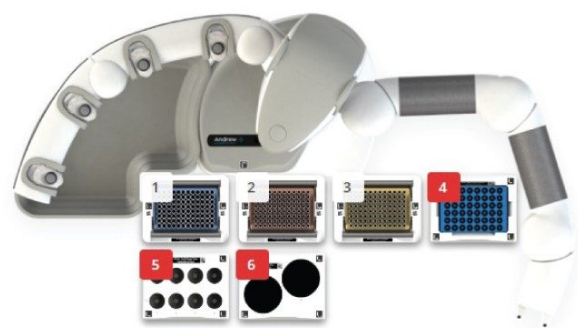
Figure 3. Andrew+ OneLab deck set up for preparation of solvent standards for calibration curve.
