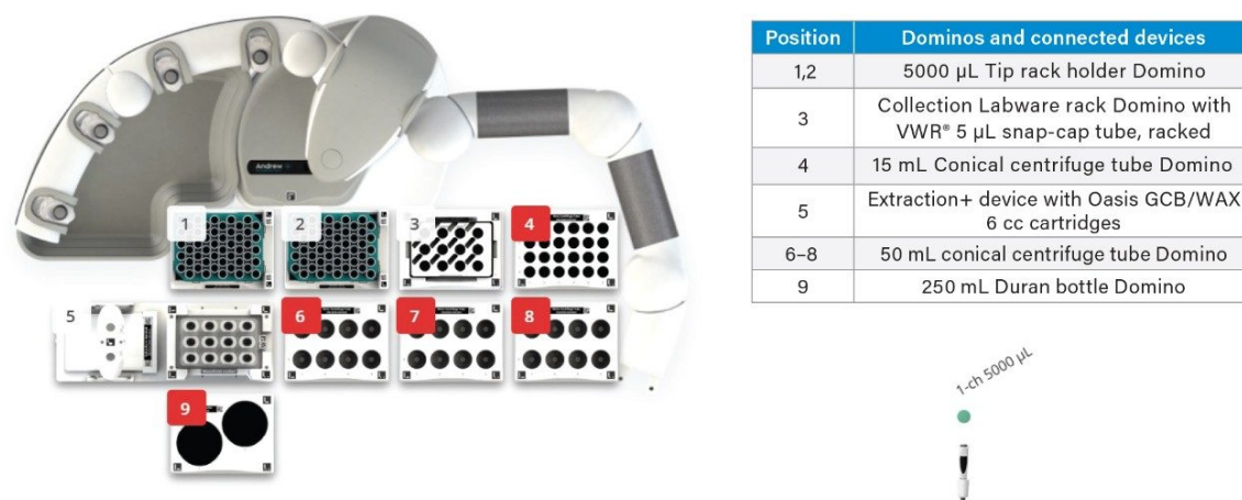
Figure 5. Andrew+ OneLab deck set up for automated PFAS extraction with Oasis WAX/GCB.
