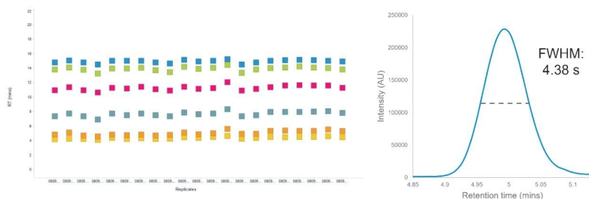
Figure 3. Retention time reproducibility of six marker peptides across injections (right). Extracted ion chromatogram of peptide VQHIQLLQK (553.8377 m/z) with the dashed line representing the full width half maximal.
