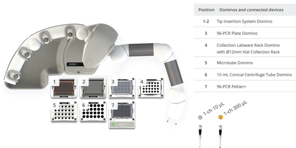
Figure 2. Top-down view of the Andrew+ Robot deck for the 8-sample RapiZyme RNases protocol. Dominos on the bench include: (1) Tip Insertion Domino with 10–300 \mu L tips, (2) Tip Insertion Domino with 0.2–10 \mu L tips, (3) 96 PCR Domino with 8-well PCR tube strip (final position for samples), (4) Collection Labware Rack Domino and 12 mm Vial Collection Rack with QuanRecovery 12 x 32 mm Screw Neck Vial 300 \mu L, (5) Conical Microtube Domino with RapiZyme MC1 or Cusativin, (6) 15 mL Centrifuge Tube Domino with 15 mL conical centrifuge tube, 96-PCR Peltier+ Connected Device with 8-well PCR tube strip (starting position for samples).
