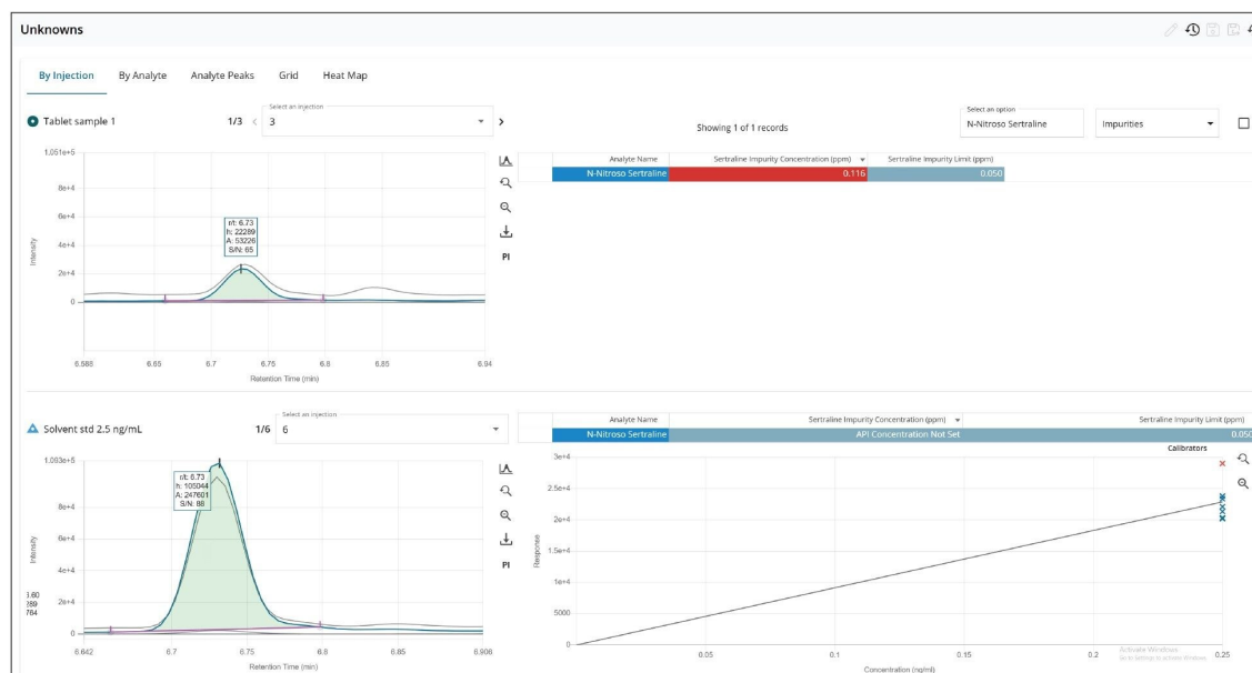
Figure 9. Unknowns page in MS Quan showing the chromatograms of N-nitroso-sertraline in tablet.
