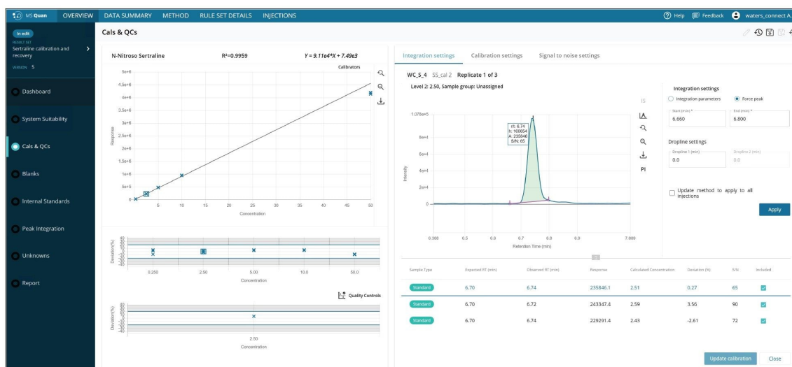
Figure 8. Linear range for N-nitroso-sertraline in solvent standards from 0.25–50 ng/mL.
