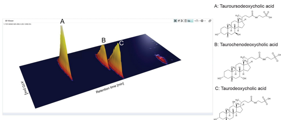
Figure 5. LC-IM of isomeric cholic acid biomarkers using resolution R \sim 250 . A:B \Delta ATD \sim 0.5 ms and B:C \Delta ATD 1.5 ms.
