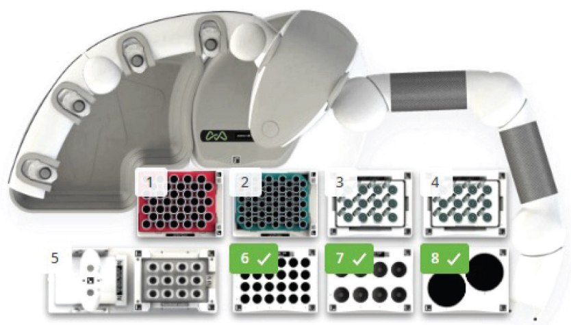
Figure 5. Andrew+ Deck Layout with Extraction+ connected device for preparation of PFAS SPE protocol using Andrew+ Pipettes and Domino Blocks: 1. Tip rack holder 10 mL; 2. Tip rack holder 5mL; 3. Collection labware rack; 4. Collection labware rack; 5. Extraction+; 6. 15 mL conical centrifuge tube; 7. 50 mL conical centrifuge tube; and 8. 250 mL glass bottle.
