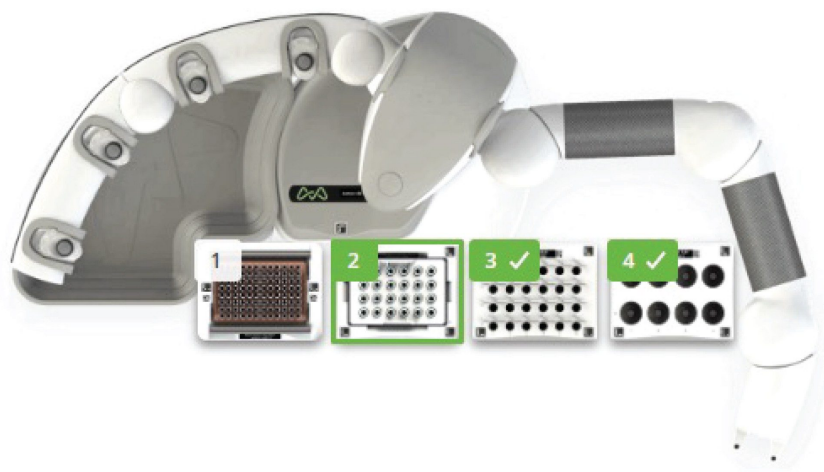
Figure 2. Andrew+ Deck Layout for preparation of PFAS internal standard calibrants using Andrew+ Pipettes and Domino Blocks: 1. Tip insertion system (10–300 µL Optifit tips); 2. Collection labware rack; 3. Microtube; and 4. Centrifuge tube.
