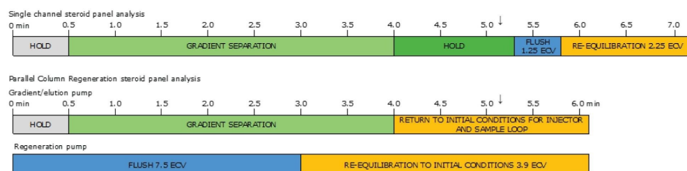
Figure 3. Timelines comparing single channel and parallel column regeneration for the chromatographic separation of prepared samples. ECV=empty column volumes. The arrow indicates the touch down point of the last eluting chromatogram peak.
