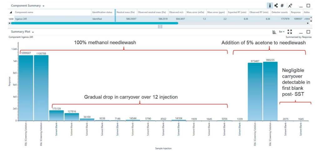
Figure 1. Effect of needle wash mix on the carry-over. Summary plot showing the removal of Irganox 245 carryover with the addition of 5% acetone to methanol needle wash.
