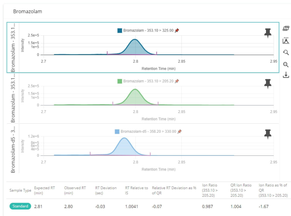
Figure 3. QUAN review peak integration review window for Bromazepam at 5 ng/mL. The quantifier, qualifier and internal standard transitions are displayed, above the acceptance criteria for retention time and ion ratio.
