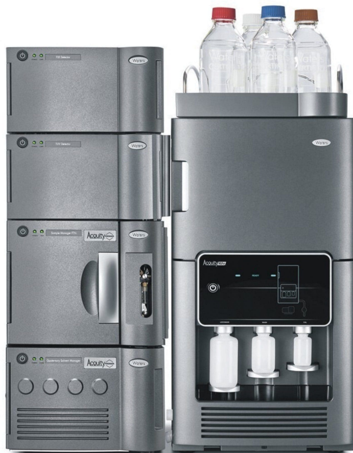
Figure 1. The ACQUITY Premier LC system coupled to the ACQUITY RDa Mass Detector.
