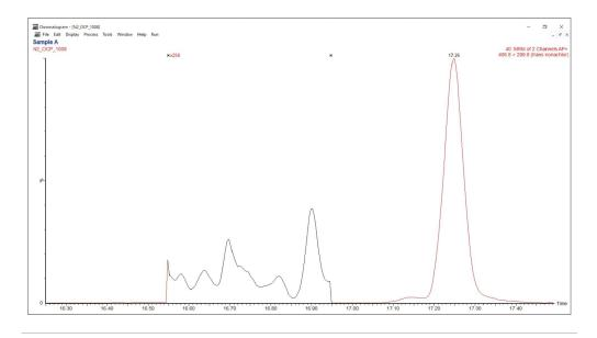
Figure 7. Trans-nonachlor at 2.52 ppb in sediment Sample A. Note baseline magnification of 250 times.
