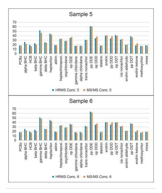
Figure 6. Concentration comparison (ppb on y-axis) between the reference method and APGC-MS/MS method using N<sub>2</sub> carrier gas.
