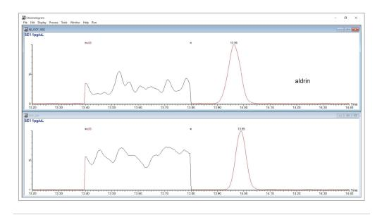
Figure 3. Aldrin APGC sensitivity comparison  $N_2$  (upper) and He (lower) carrier gas for 1 ppb (1 µL at 1 pg/µL = 1 pg mass-on-column).
