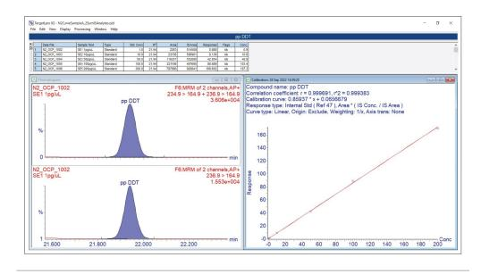
Figure 5.  $N_2$  carrier gas calibration curve example for p,p DDT with 1 ppb
