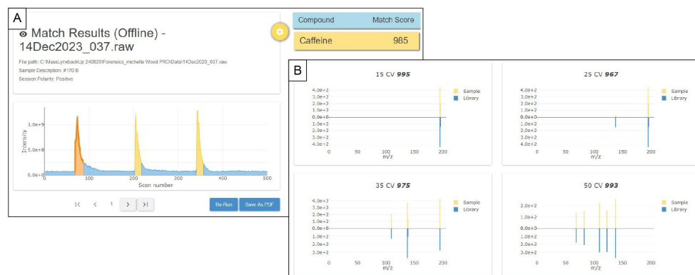
Figure 3. LiveID analysis of a seized sample. Panel A shows three “dip and detect” replicates for the sample and the match score 985 (maximum 1000) obtained for the first replicate. Panel B displays the detail for this spectral match; all four cone voltages are used in the identification process with the weighted mean (lowest cone voltage with the highest weighting) used.
