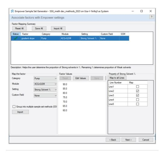
Figure 7. Empower SSG for creation of chromatographic methods for optimization of gradient slope. Gradient slope mapped to pump and strong solvent percentage, applied to lines 2 and 3 in the gradient separation.
