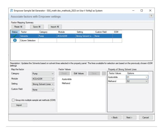
Figure 3. Empower SSG. Settings for organic solvents: pump and strong solvent lines.
