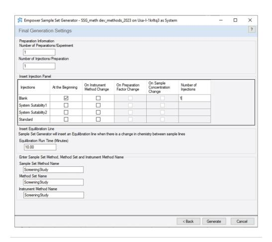
Figure 5. Empower SSG. Final settings for generation of chromatographic method including sample preparation information, injection panel (blank, system suitability, standard), equilibration time, and names for the methods.
