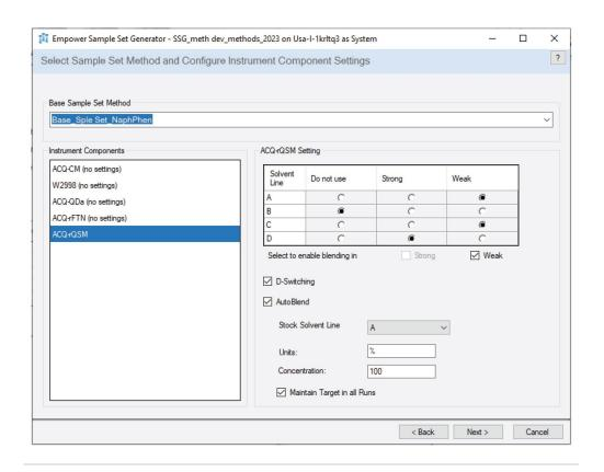
Figure 2. Empower SSG. Load base sample set method and configure instrument components settings as required. ACQUITY rQSM pump setting: strong and weak solvent lines, D-switching for strong solvent, and AutoBlend with stock solvent line A.
